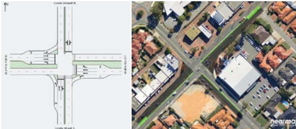
Figure 11-15 Walter Road West/ Coode Street – Mitigated Geometry
