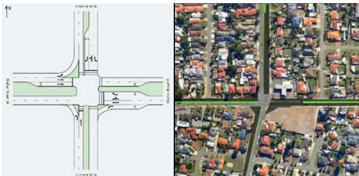
Figure 11-7 Walter Road West/ Crimea Street – Mitigated Geometry
