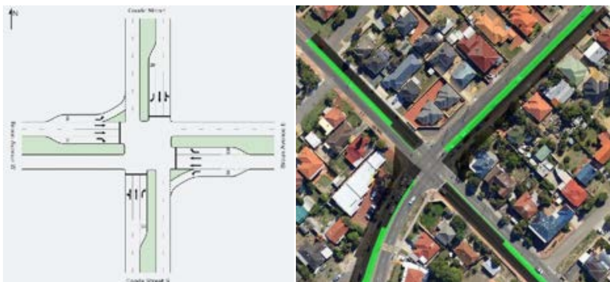
Figure 11-1 Broun Avenue /Coode Street – Mitigated Geometry
