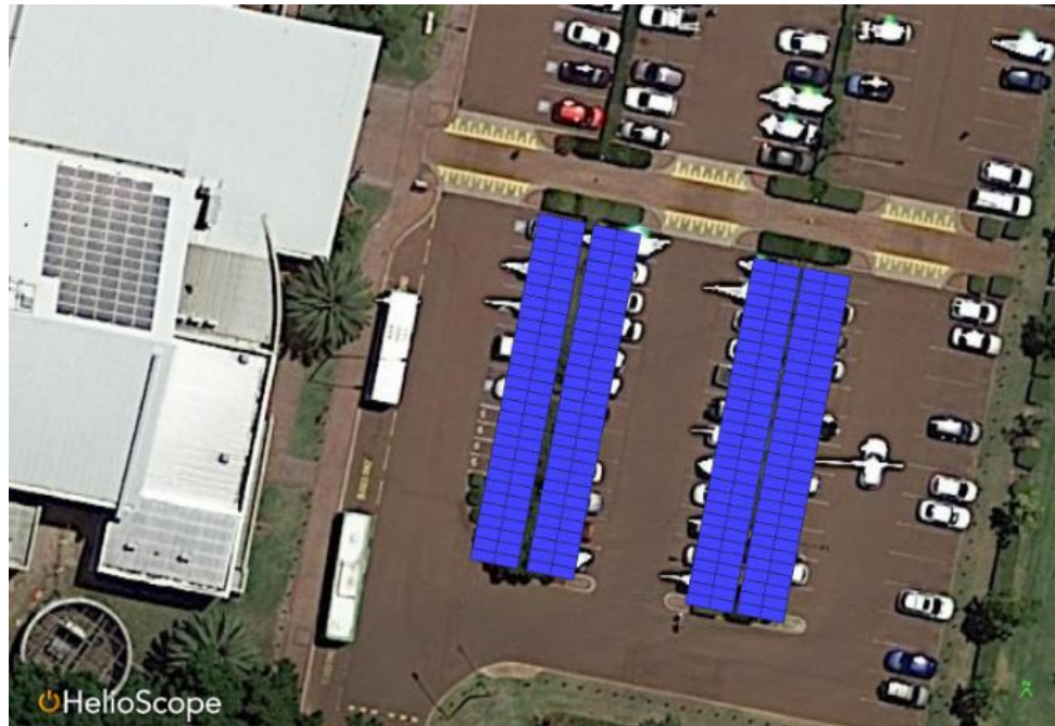
FIGURE 32: BAYSWATER WAVES STAGE 3 – MODELLED +99.6 kW OF CARPORT SOLAR
