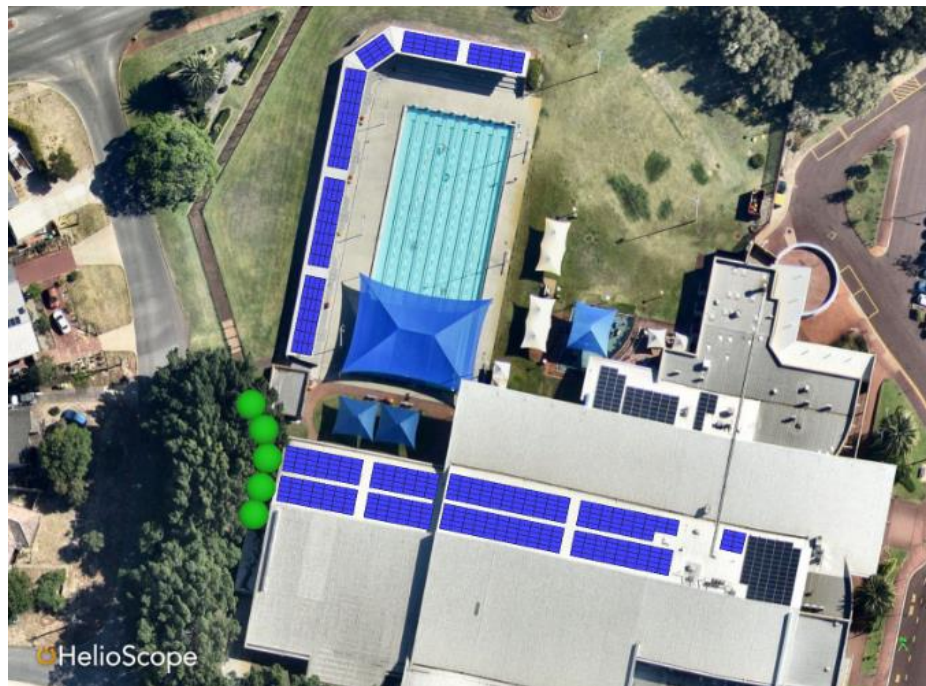
FIGURE 31: BAYSWATER WAVES STAGE 2 – 140.7 kW OF SOLAR PV ON ROOFS INCL. THE GRANDSTAND
