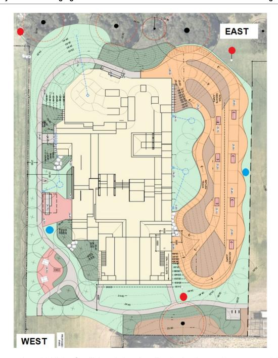
The image above highlights floodlight pole locations illuminating the previous soccer training site now to become the new skate and BMX facility. Three original existing columns and lamps shown in red are providing 50 lux illumination to the site. Two (2) additional new poles are proposed and shown in blue in order to increase illumination and provide a more balanced illumination across the skate and BMX area.
