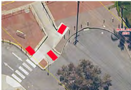
Image 4 Kerb ramps installed at Coles Maylands.
