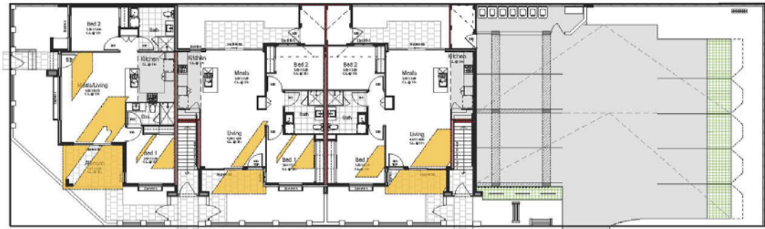
GROUND FLOOR SOLAR ACCESS DIAGRAM - JUNE 21st @ 1pm 1:200
