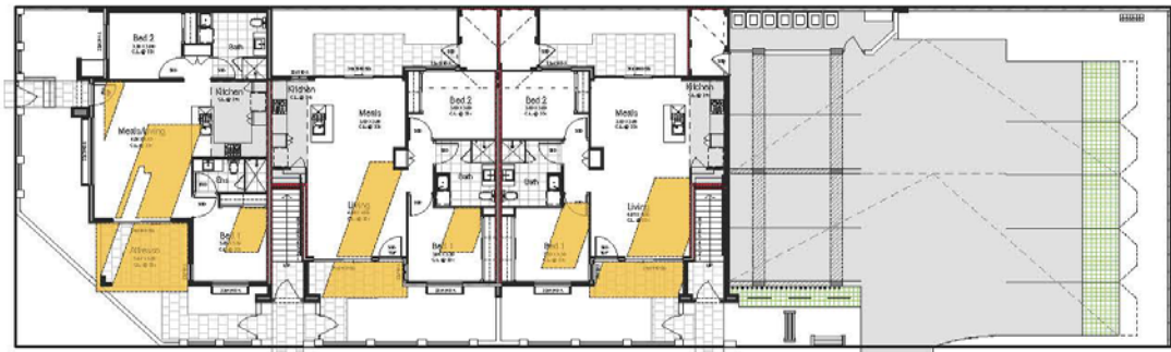
GROUND FLOOR SOLAR ACCESS DIAGRAM - JUNE 21st @ 2pm 1:200
