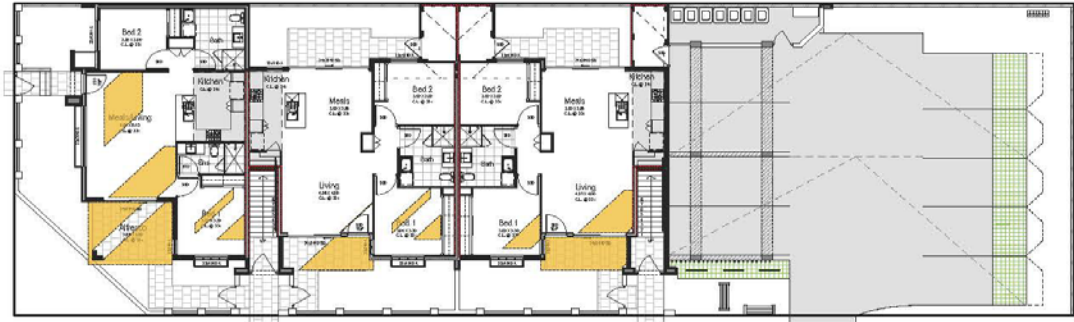
GROUND FLOOR SOLAR ACCESS DIAGRAM - JUNE 21st @ 12pm 1:200
