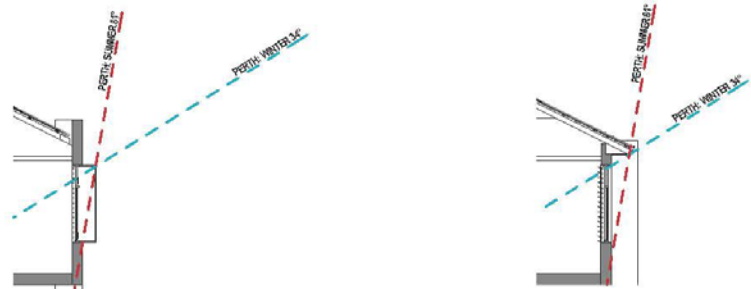
WINDOW SHADING WITH 300mm SURROUND 1:100
