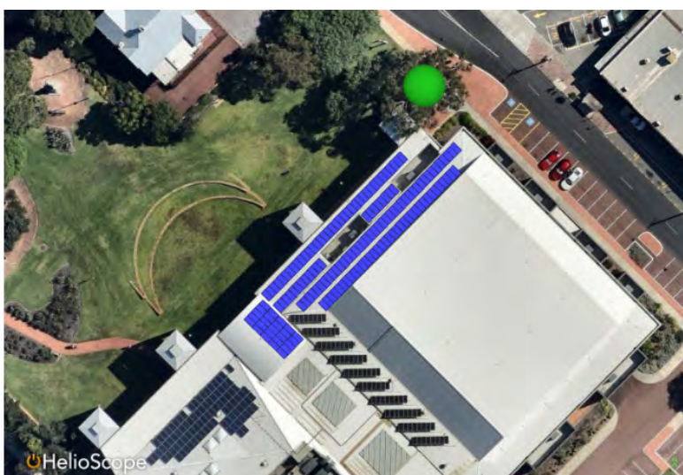
FIGURE 33: THE RISE STAGE 1 – MODELLED 65.2 kW OF SOLAR PV ON ROOFS
