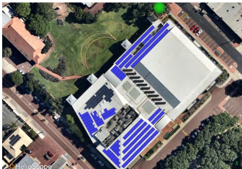
FIGURE 34: THE RISE STAGE 2 – MODELLED +116.6 kW OF SOLAR PV ON ROOFS
