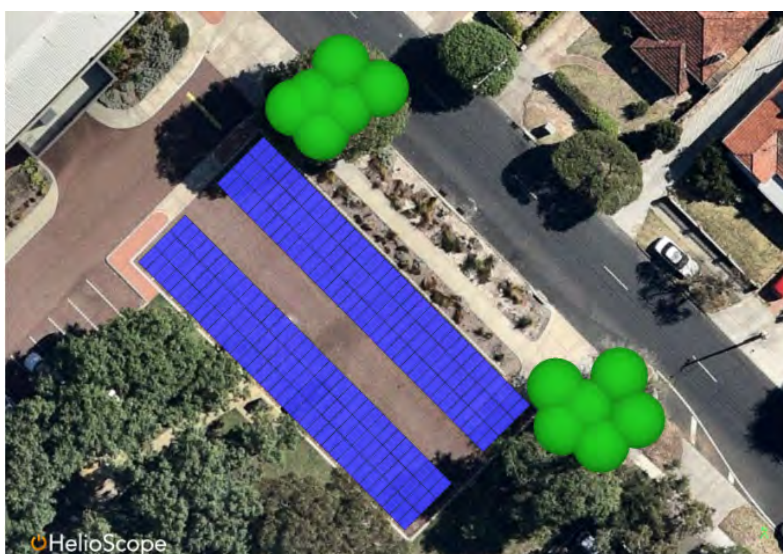
FIGURE 35: THE RISE STAGE 3 – MODELLED +87.2 kW OF CARPORT SOLAR
