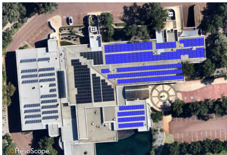
FIGURE 36: CIVIC CENTRE STAGE 1 - MODELLED +150.2 kW ADDED ROOFTOP SOLAR
