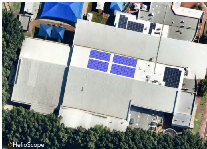
FIGURE 30: BAYSWATER WAVES STAGE 1 – MODELLED 59.3 kW OF SOLAR PV ON ROOFS
