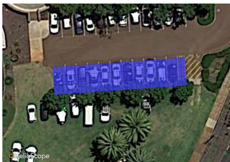
FIGURE 37: CIVIC CENTRE STAGE 2 - MODELLED +36.1 kW OF CARPORT SOLAR
