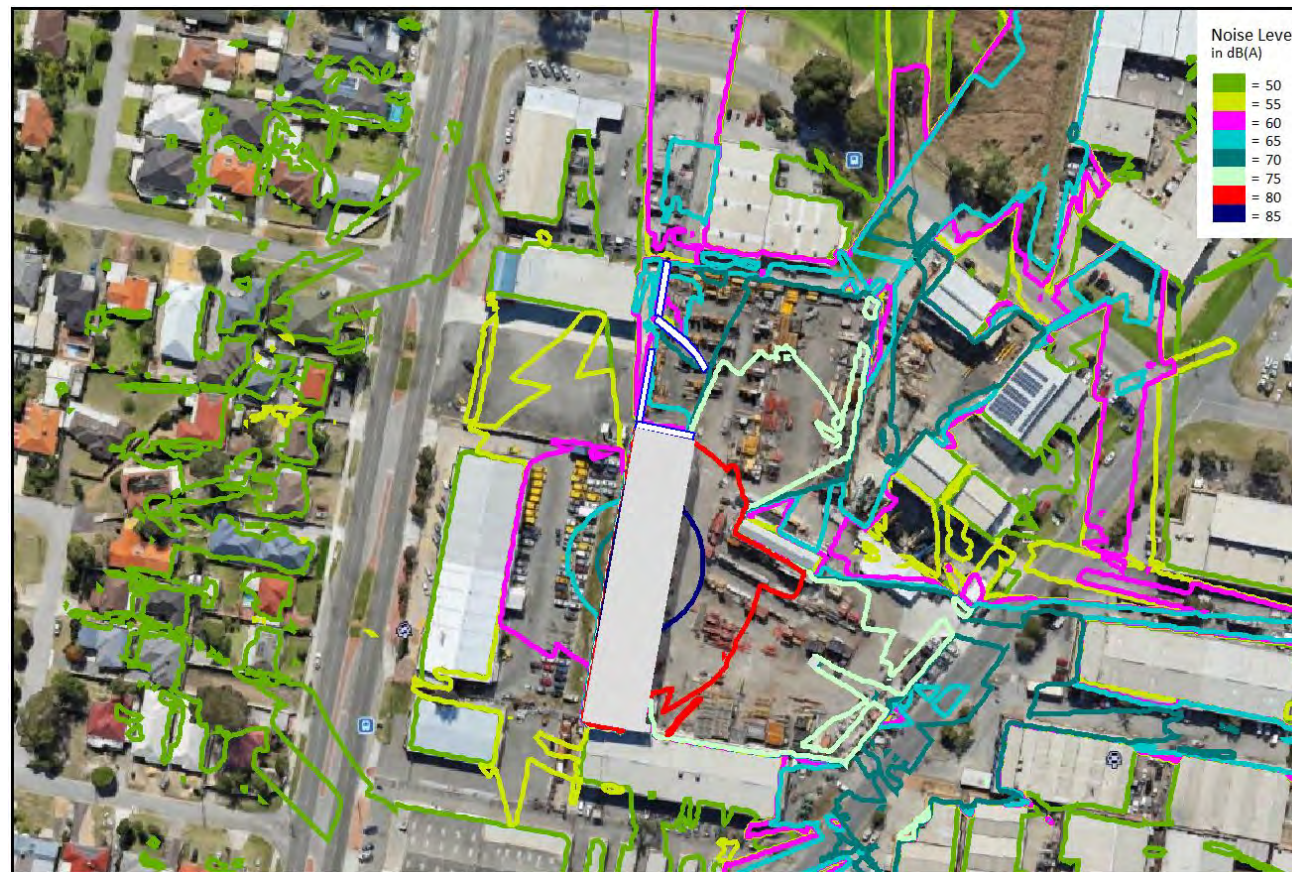
Figure 9: Worst-case noise level L_{A\text{Max}} contours for scenario 3.
