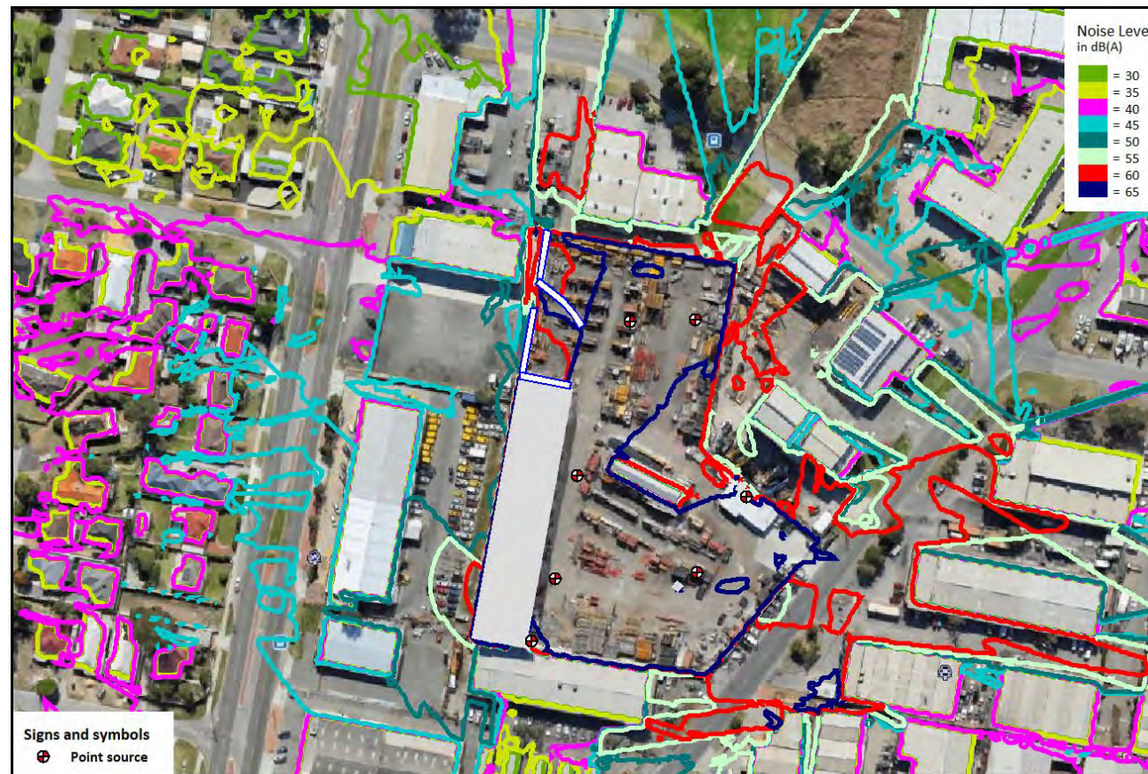
Figure 15: Worst-case noise level contours for scenario 9.
