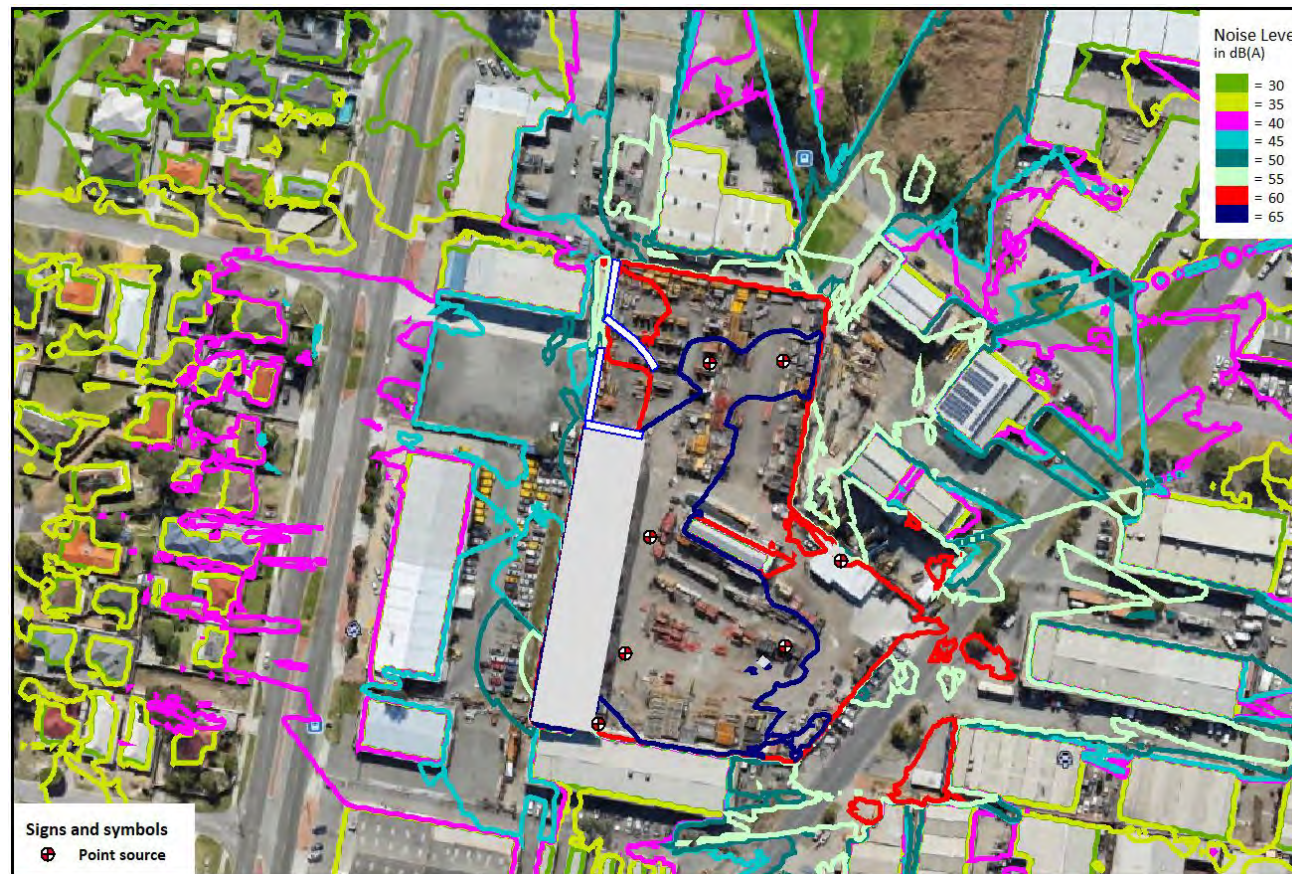
Figure 7: Worst-case noise level contours for scenario 1.
