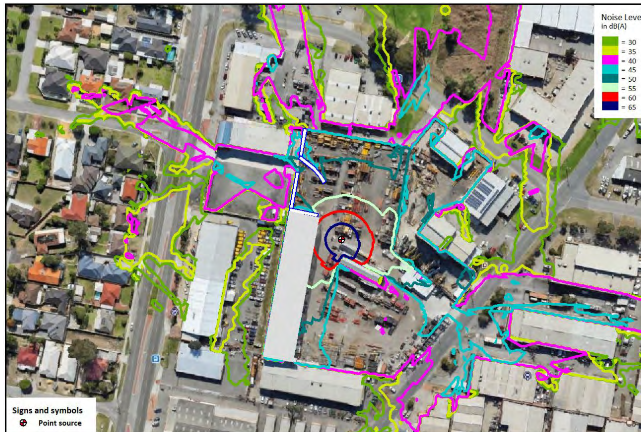
Figure 11: Worst-case noise level L_{A\text{Max}} contours for scenario 5.
