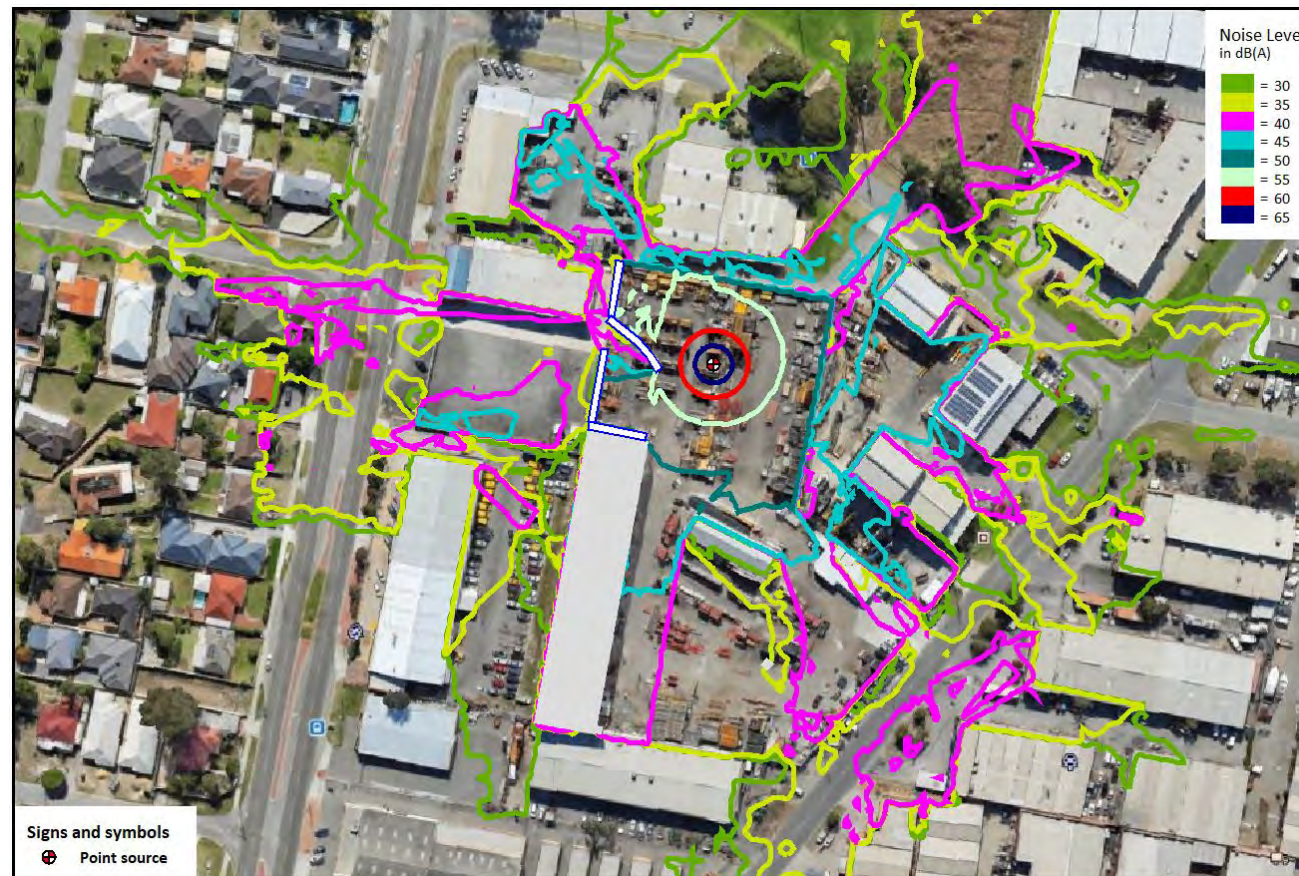
Figure 14: Worst-case noise level contours for scenario 8.
