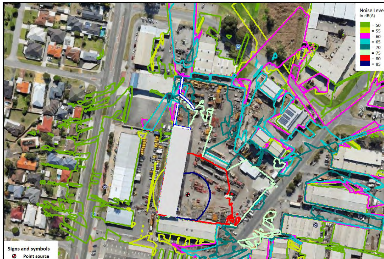
Figure 13: Worst-case noise level L_{A\text{Max}} contours for scenario 7.
