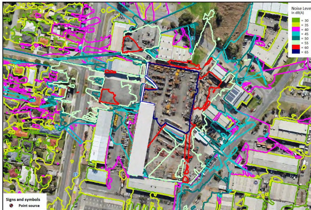
Figure 10: Worst-case noise level L_{A\text{Max}} contours for scenario 4.
