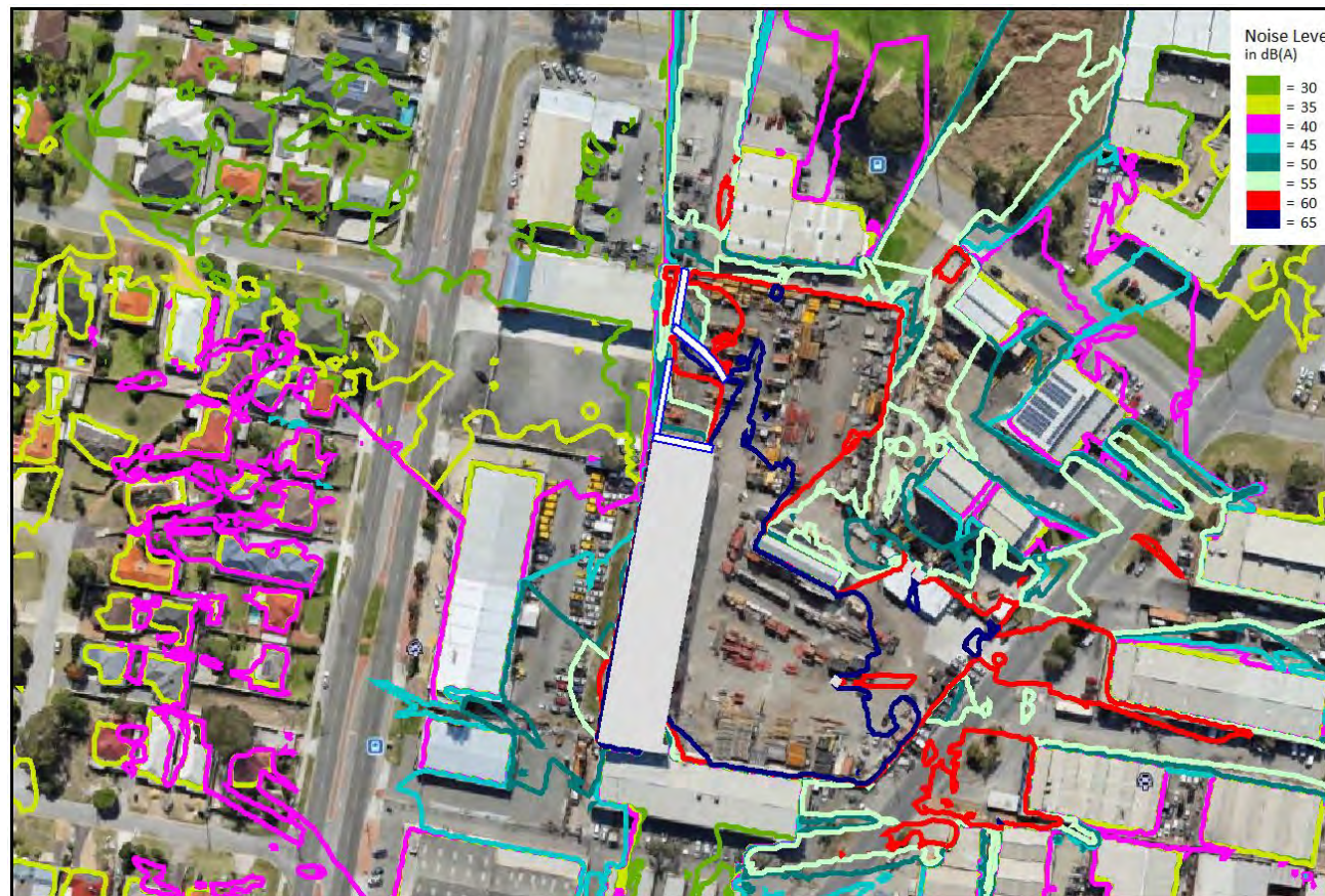
Figure 12: Worst-case noise level contours for scenario 6.
