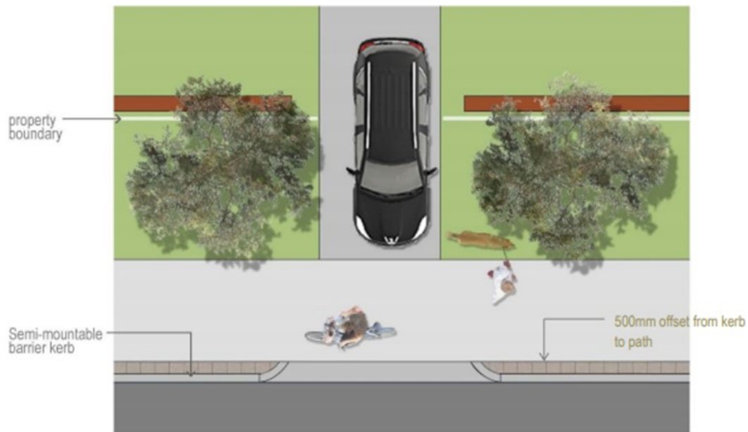
Figure 7 Plan View of Model Crossover Design
