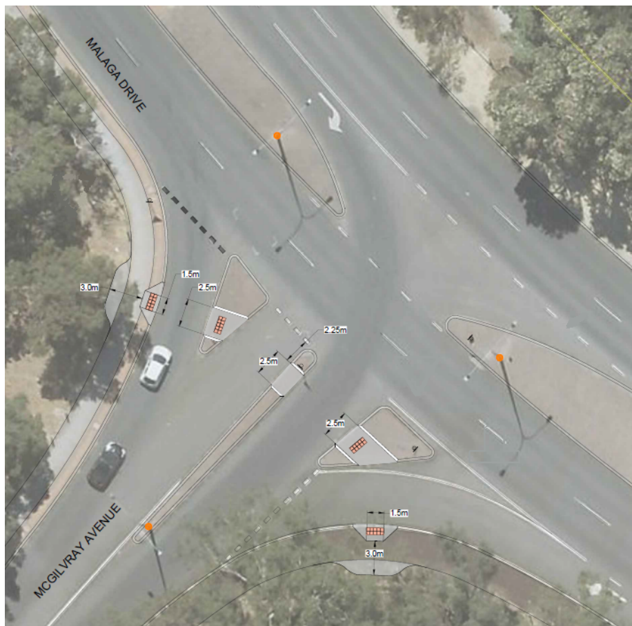
Image 1: Pedestrian ACROD Compliant Crossing Facilities across McGilvray Avenue, Noranda.
