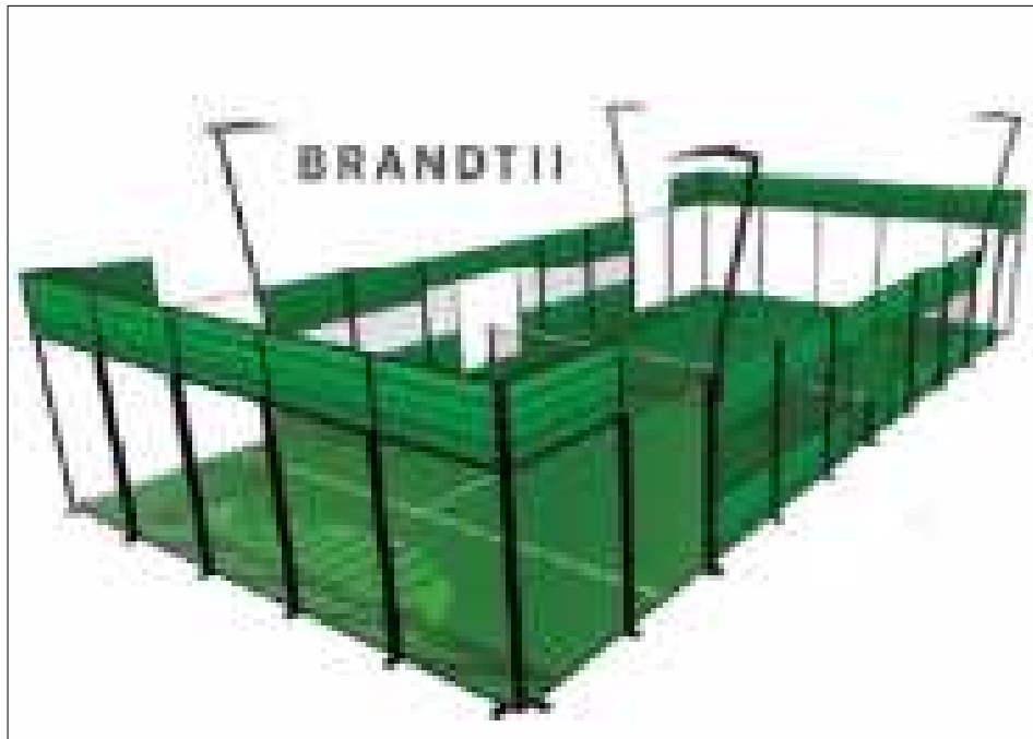
FIGURE G3 – IMAGE OF A PADEL COURT FITTED WITH THE ACOUSTIC PANELS PRIOR TO ADDITION OF THE ACOUSTIC BARRIERS
