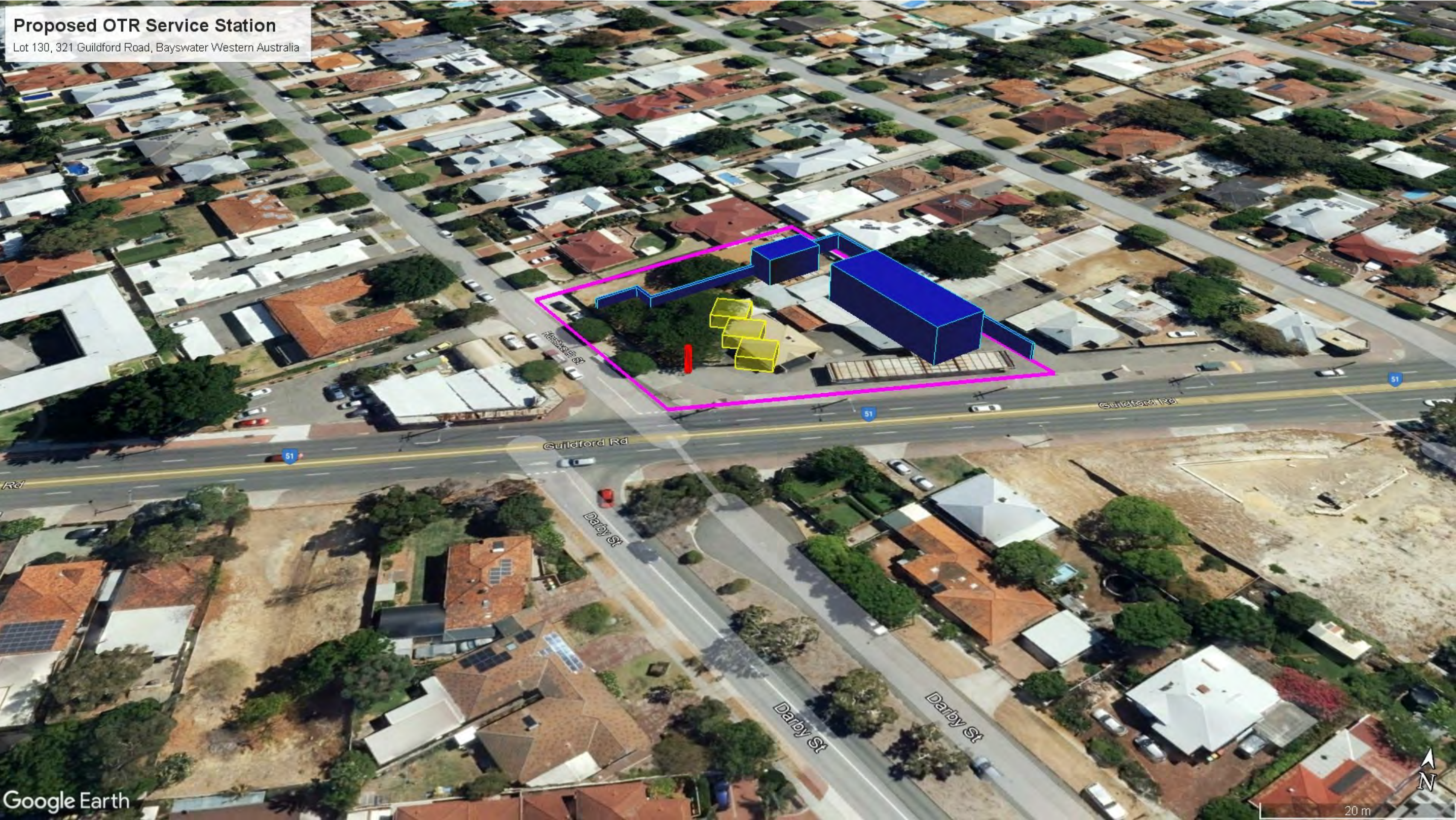
Figure 1-2: Modelling Depiction of Proposed Service Station – Blue (Station POS Building & Site Perimeter Brick Walls), Red (Bulk Tank Vents), Yellow (Refuelling Bowsers)
