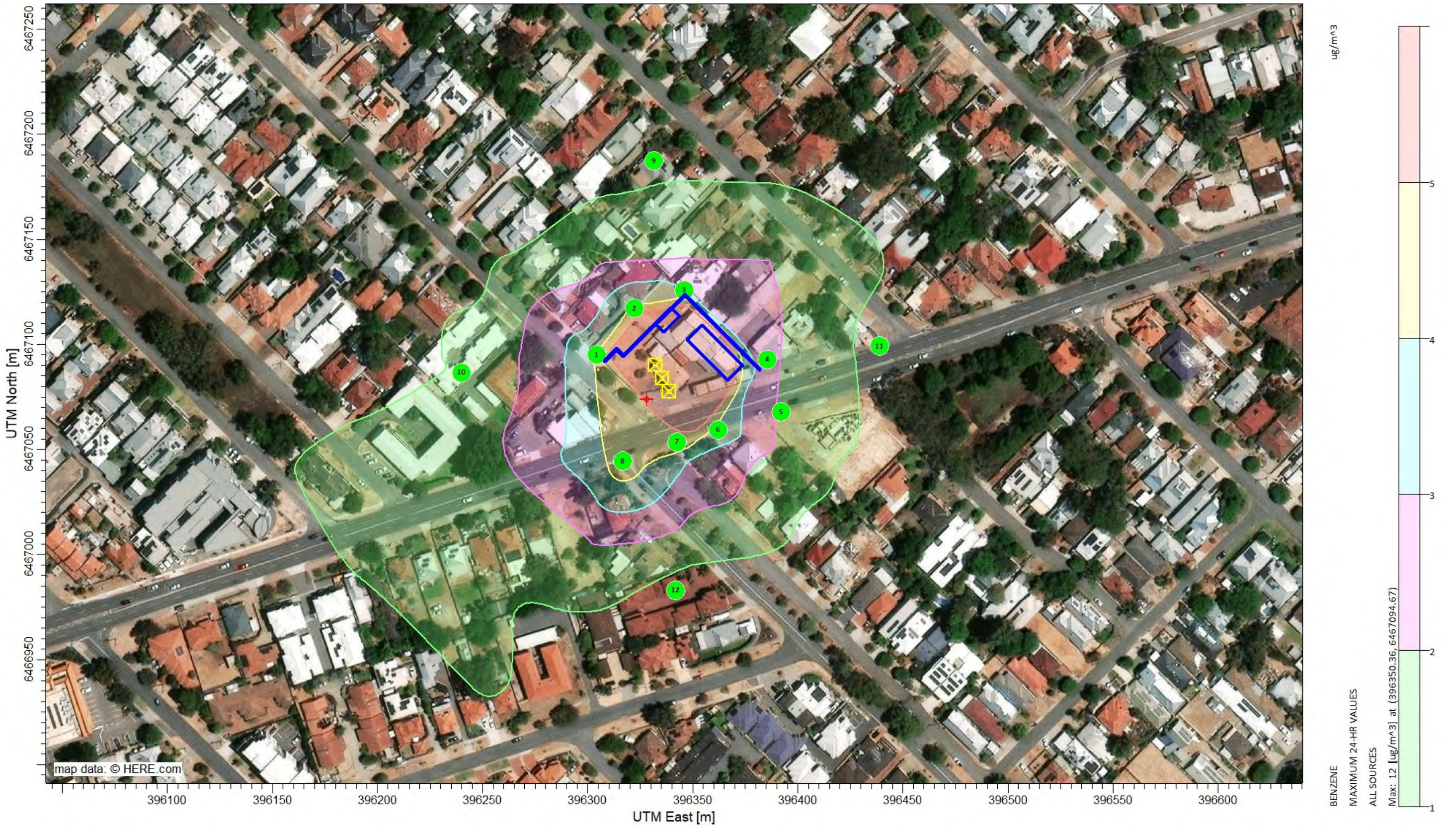
Figure 3-2: 24 Hour Benzene Predicted Ground Level Concentrations (VR1 & VR2)
